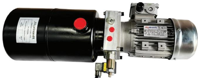
This unit is specifically designed for dock leveller applications, with full hydraulic control.
